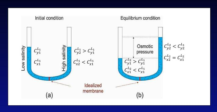
Partition Coefficient  $\Phi = \Delta C_y / C_{y2}^{L_1} \Delta C_y = C_{y2}^{L_1} - C_{y2}^{L_2}$
