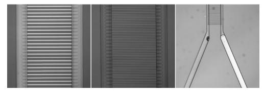
Figure 12 – Three images taken during the vaporization of the ternary mixture in the chip. Left: Micro- and nanochannels filled with air; Middle: Micro- and nanochannels filled with the ternary hydrocarbon mixture; Right: Vaporization of the ternary mixture stopped in one of the microchannels at 345 °K.
